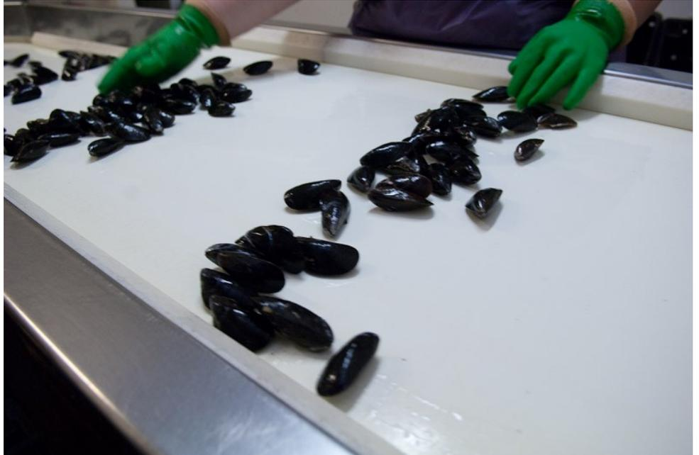
**Figure 4: Mussels being graded during processing**
